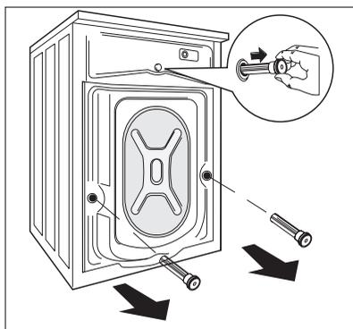
5. Fill the smaller upper hole and the two large ones with the corresponding plastic plug caps supplied in the bag containing the instruction booklet.
